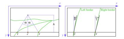
*Left:* Model visualization for the perspective image: Center point c defines at fixed height h angle  $\alpha$  which identifies left and right lane border points at l and r
