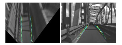
*Left*: Generated points  $(I_n, y_n)$  and  $(r_n, y_n)$  using the described method (in yellow) and an extended method where each particle is defined by 2 rows backward and 8 rows forward (in cyan), defining an  $11 \times 4 = 44$ -dimensional particle space
