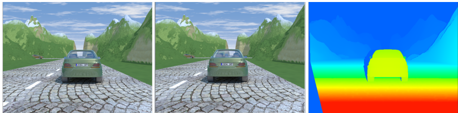
Figure : Stereo image pair with a ground truth (color-coded) disparity map.
