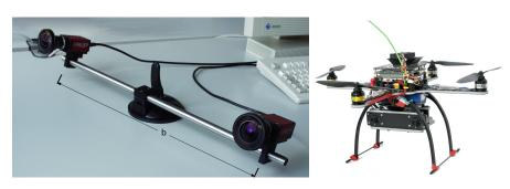
Left: A stereo camera rig on a suction pad with indicated base distance b Right: Stereo camera system integrated into a quadcopter
