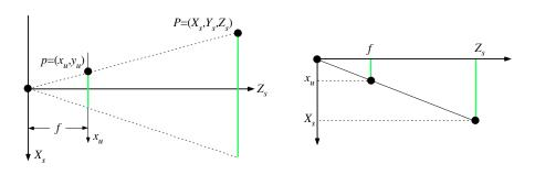
Left: Central projection in the  $X_sZ_s$  plane for focal length f
