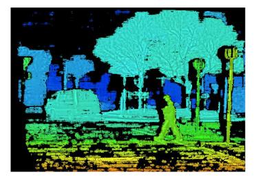
Color: Color-encoded disparity values at pixel locations Black: Pixel location without assigned disparity value
