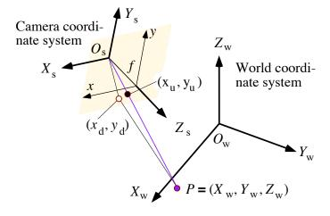
$x_d$  and  $y_d$  are distorted (by lens distortion) coordinates in the image
