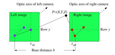
We describe each camera by using the model of a pinhole camera
