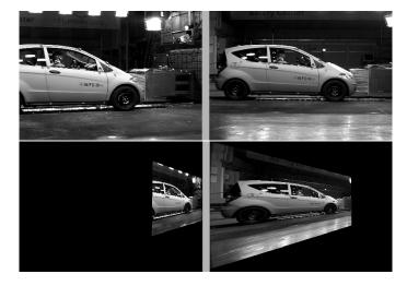
Recorded pair of images before and after rectification Recording:  $b \approx 10$  m, different viewing directions, definitely not CSG
