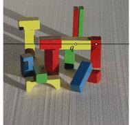
Corresponding point q to a point p in left image is left of this point in the right image
