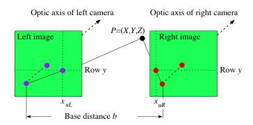
This process is called *geometric rectification*; it can be done by using intrinsic and extrinsic parameters as obtained by camera calibration
