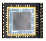
Edges of individual sensor cells (phototransistors) are  $1.4\mu m$  to  $20\mu m$
