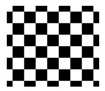
2D checkerboard pattern as commonly used for camera calibration the corners of squares are the calibration points
