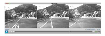
Three cameras installed with goal to match canonical stereo geometry Base distances: left to middle:  $\approx$ 40 cm, middle to right:  $\approx$ 30 cm
