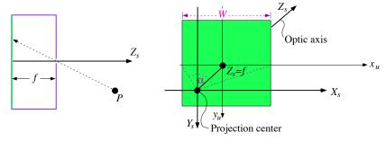
Left: Sketch of an existing pinhole camera ("shoebox camera") Point P projected onto an image plane at distance f behind the hole
