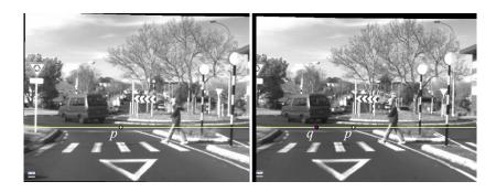
Start at p and search along the epipolar line for a corresponding q How to detect q?
