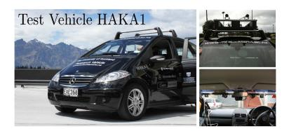
Examples of mounted cameras inside or on top of the vehicle
