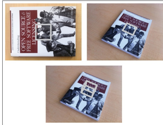
Figure 2: Example of computing the projection matrix for a new view using a planar object as marker. Matching image features to an aligned marker gives a homography that can be used to compute the pose of the camera. Template image with a gray square (top left); an image taken from an unknown viewpoint with the same square transformed with the estimated homography (top right); a cube transformed using the estimated camera matrix (bottom).
