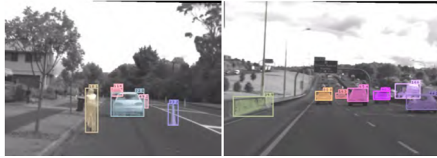
Figure 3: Mean distances to segmented objects. Left: Distances to objects within the lane area only. Right: Distances to all the detected objects.
