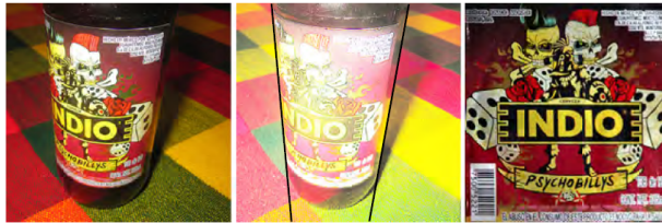
Figure 1: Left: Example of an input image of a cylindrical shape with glued-on label. Middle: Approximate location of occluding contours of cylinder, generated by manual interaction. Right: Extracted flat label from multiple input images.
