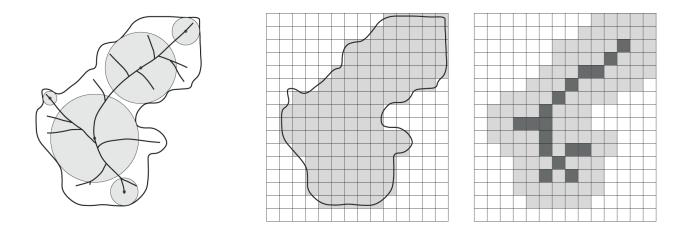
Left: a set in the Euclidean plane and its medial axis. Middle: the Gauss digitization of this set at some grid resolution. Right: illustration of an expected outcome when calculating the medial axis. The chosen grid resolution restricts the complexity of the medial axis. In the real plane, any cavity "splits" the medial axis into two branches.
