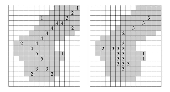
Medial axis transforms for distance transforms ( $d_4$  and  $d_8$  as shown in Lecture 08 for this set). Left:  $d_4$ . Right:  $d_8$ .
