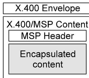
X.400 security required using (and trusting) an X.400 MTA; MSP requires only trusted endpoints
