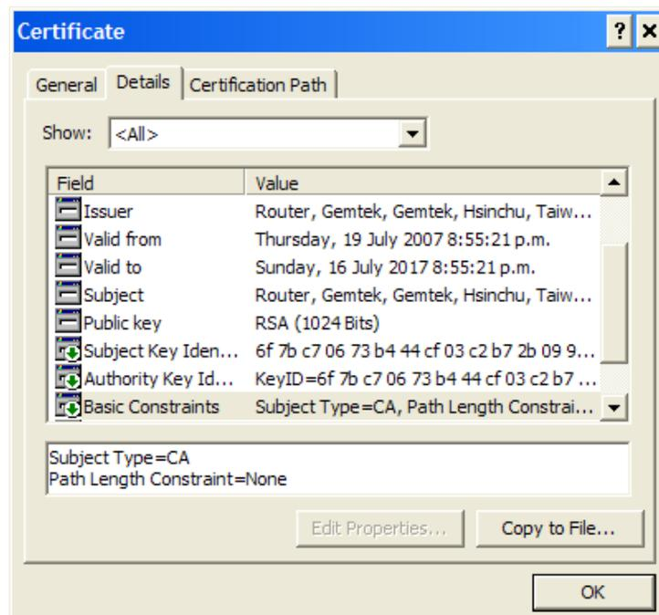
**Figure 95: Embedded device certificate that's also a root CA**
