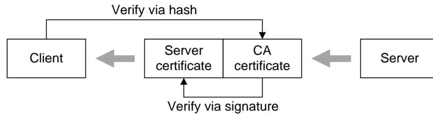
**Figure 189: Simple certificate checking for mobile client applications**
