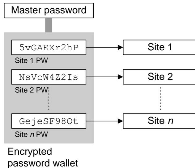
**Figure 171: Password diversification using a password wallet**
