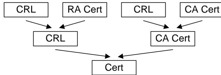
**Figure 185: CRL-based revocation checking for a chain of length 3**
