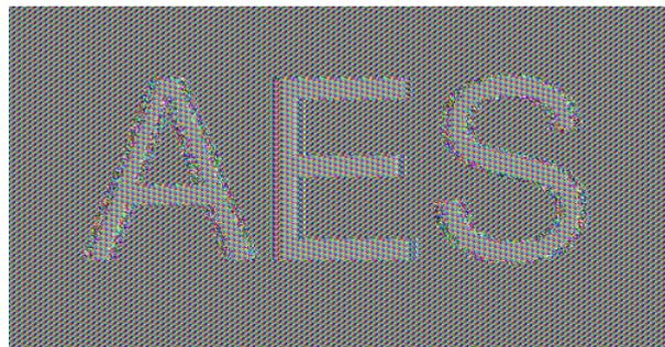
**Figure 96: Original image data (top) and the same data encrypted with AES-256 in ECB mode (bottom)**
