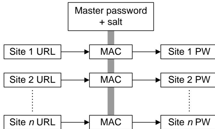
**Figure 172: Password diversification using hashing**
