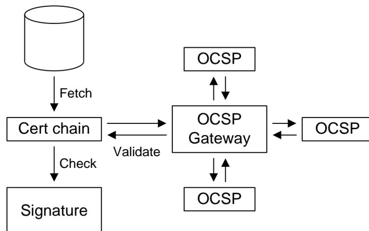
**Figure 187: Offloading the revocation checking process**
