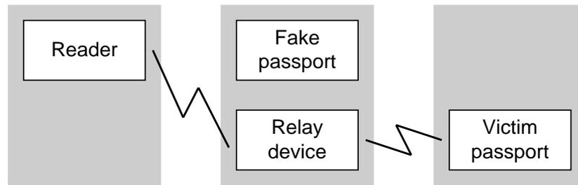
**Figure 130: Relay attack on a contactless interface**
