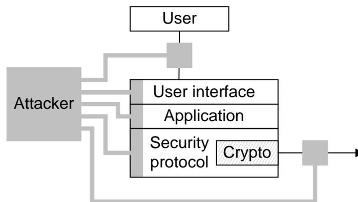
**Figure 67: Cryptography is something to be bypassed, not attacked**
