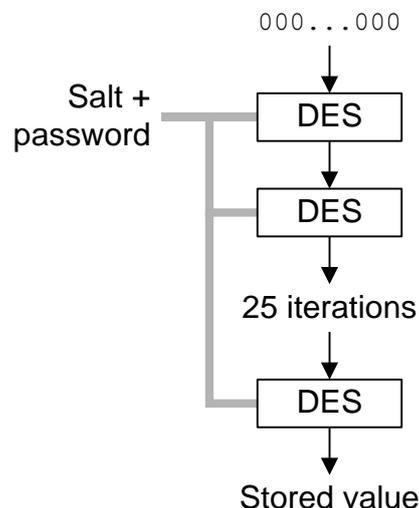
**Figure 160: Unix stored-password protection**
