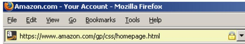
**Figure 136: Unambiguous security indicators for SSL**
