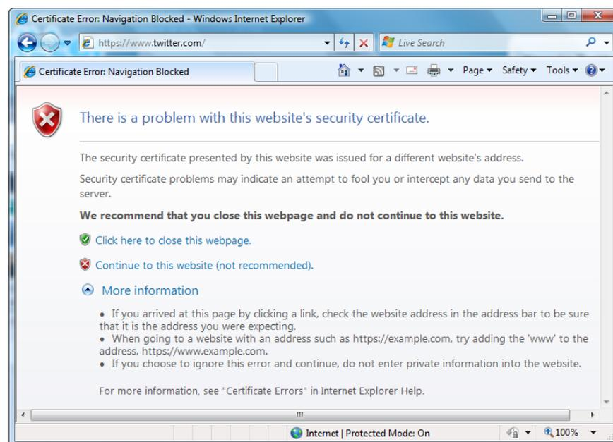
**Figure 4: Normal errors when accessing an HTTPS web site**
