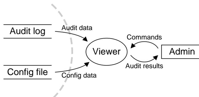
**Figure 73: Data flow diagram for a security audit application**
