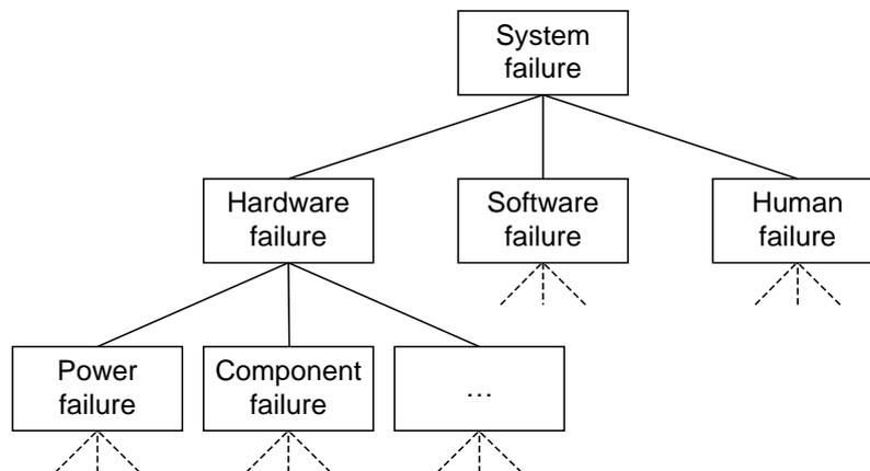
Figure 70: Fault tree analysis
