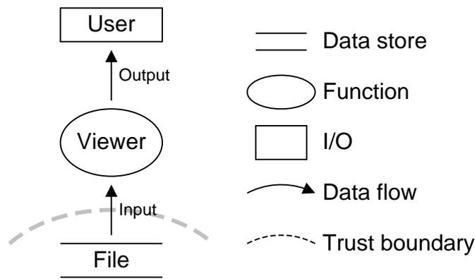
**Figure 72: Data flow diagram for an image viewer**
