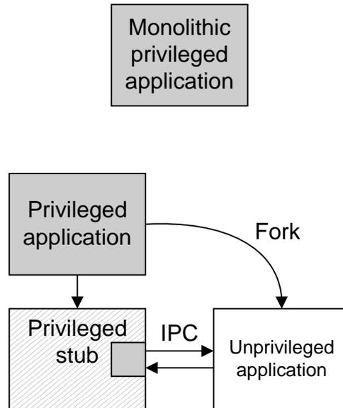
**Figure 90: Monolithic privileged application (top) vs. privilege-separated application (bottom)**
