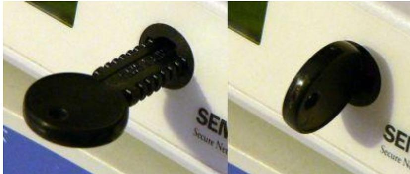
**Figure 128: A Datakey being used to key a VPN box**
