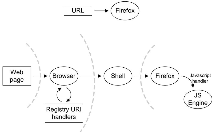
**Figure 76: DFD for presumed (top) and actual (bottom) Firefox URL handling**
