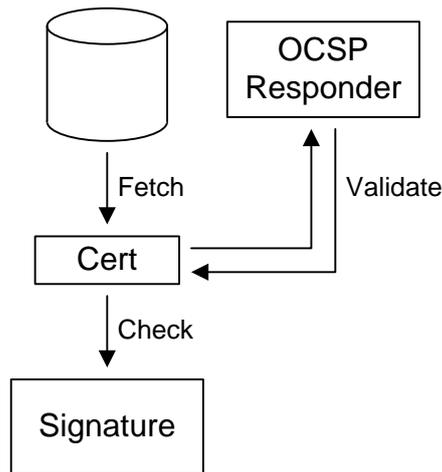
**Figure 186: Certificate usage model with OCSF responder**
