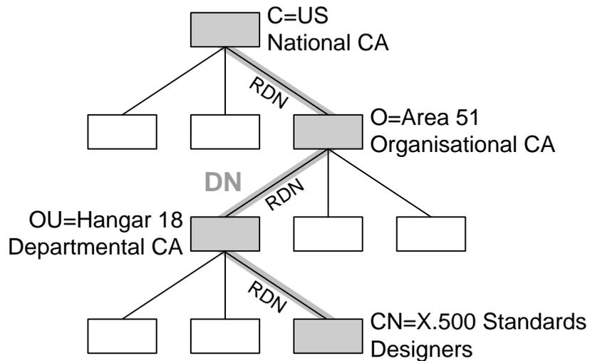
**Figure 176: X.500 directory with certificate-based access control**
