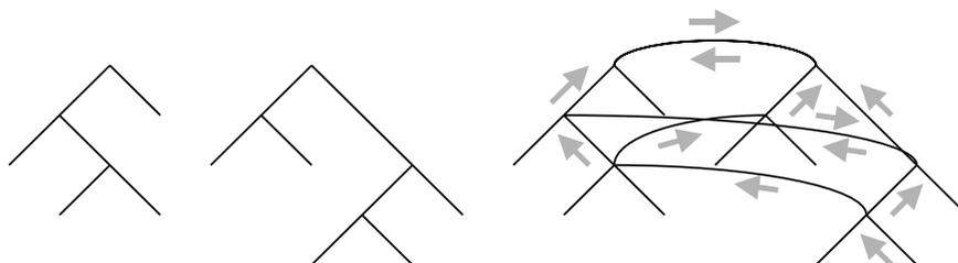
**Figure 182: Certificate hierarchy (left) with cross-certification (right)**
