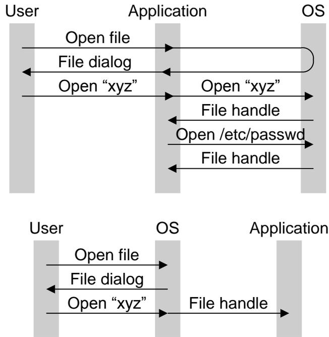
**Figure 92: Standard excess-authority file open (top) vs. security by designation (bottom)**
