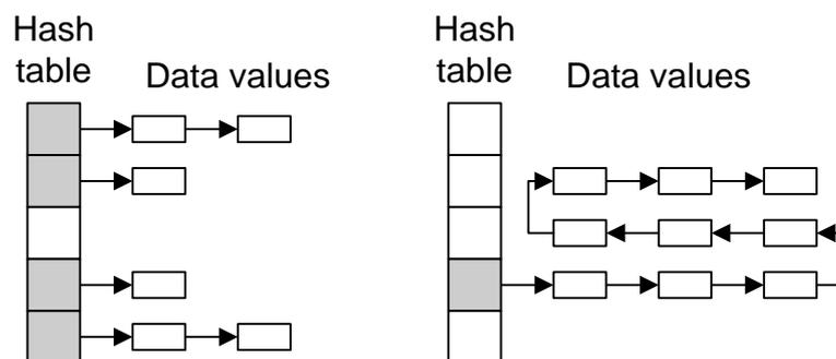
**Figure 82: Hash table in the presence of normal (left) and malicious (right) data**
