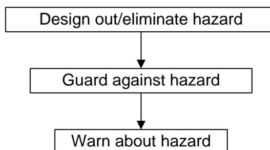
**Figure 8: The safety engineering hazard control hierarchy**
