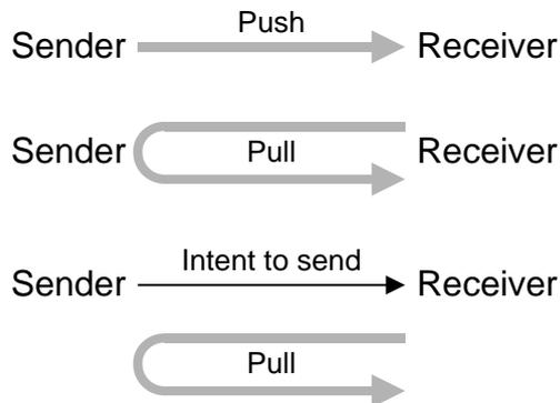
**Figure 81: Push vs. pull content distribution**
