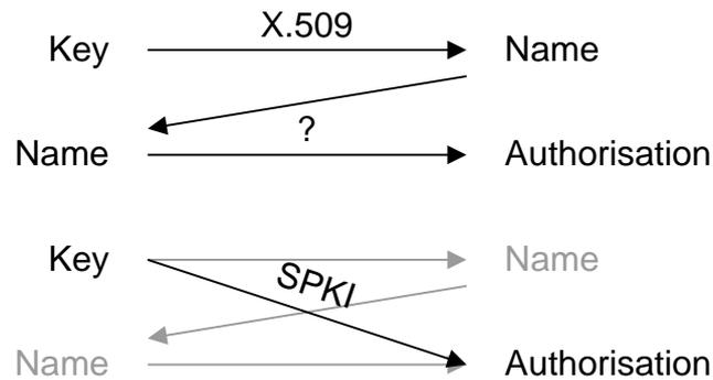
**Figure 179: X.509 (top) and SPKI (bottom) certificate functionality**
