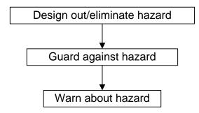
Figure 8: The safety engineering hazard control hierarchy
