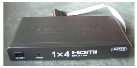
Figure 106: HDMI switch/HDCP stripper
