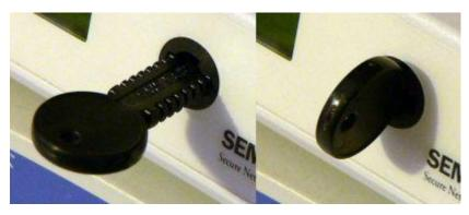
Figure 128: A Datakey being used to key a VPN box
