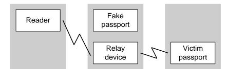
Figure 130: Relay attack on a contactless interface
