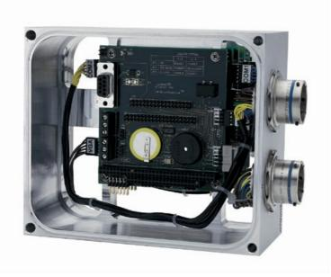
Figure 10: HiDAN embedded PC internals (image courtesy RTD)
