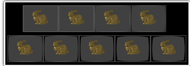
Fig. 13 One input image of the data sets D1 to D9, demonstrating the effect of adding an increasing amount of barrel distortion
