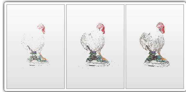
Fig. 1 Several SfM stages of the reconstruction of our White Rooster data set. Left the initial two-frame reconstruction. Middle an intermediate stage after 22 images have been added. Right the final construction with 39 images
