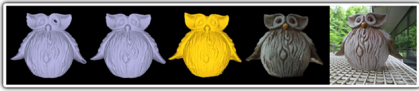
Fig. 17 From left to right model obtained with laser scanner before and after filling holes, model obtained using our image-based modeling system before and after texture reconstruction, and a photograph of the original model
