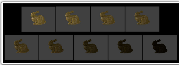
Fig. 10 Brightness of input images for the test data sets testing the relationship between image brightness and reconstruction quality
