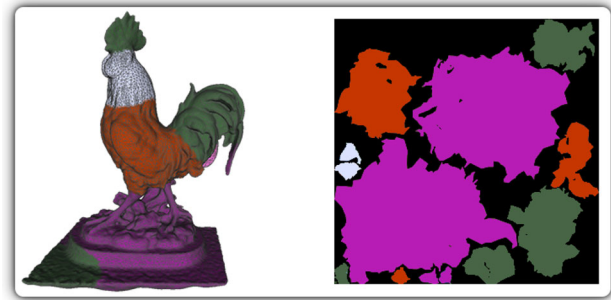
Fig. 3 Our white rooster model segmented into patches ( left ) and the corresponding regions in the texture atlas ( right )
