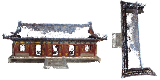
Figure 1: 3D point clouds of a historic building using an image-based modelling technique with 21 input images.
