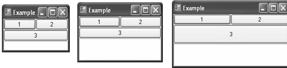
Figure 12: Example layout with linear constraints and penalty constants, adjusted to window resizing.
