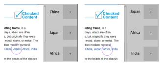
Figure 1. Existing Multiple Confirm click alternative: confirm buttons are unstable as the dwell position changes, even if referring to the same link (left vs. right).
