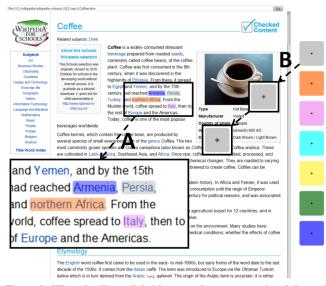
Figure 2. When dwelling, clickables near the gaze are colored dynamically (A) and associated with stable confirm buttons (right margin). The crosshair of a confirm button is animated during dwell (B).
