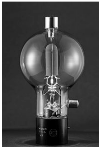
An RCA Triode valve or vacuum tube
