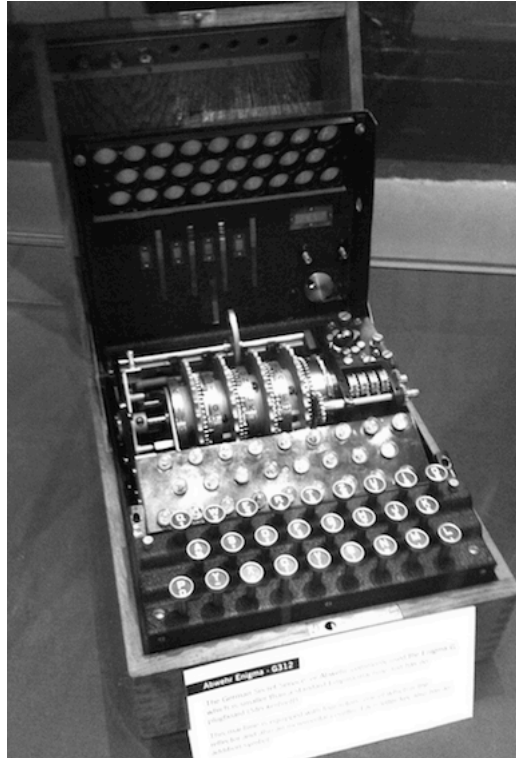
An Enigma Machine showing the rotors
