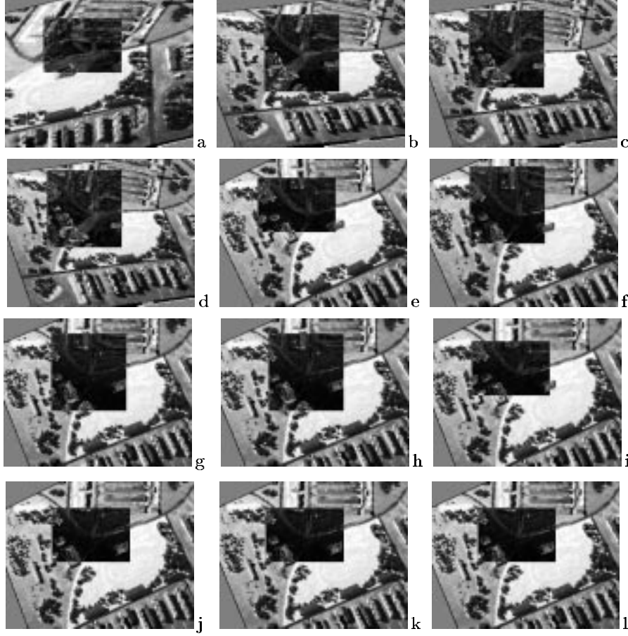
Fig. 5. Next-to-top image M15 affinely adjusted to M28 using the affine parameters in Table 2. The dark rectangles show positions of the prototypes and the grey-coded values of the residual pixel-wise errors for the least square correlation matching.
