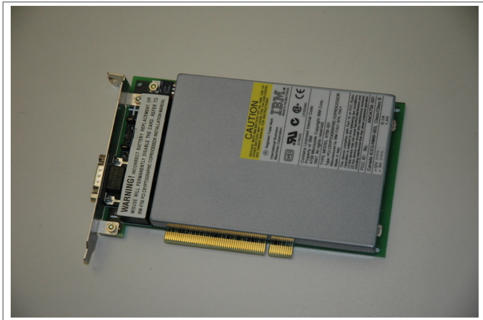
Figure 3.4: Photograph of the IBM 4758 secure coprocessor.
