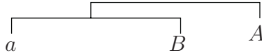
Fig. 8. Multiplication by 2. Here a represents the input; A represents the output. The machine computes 2a . The combined weights of a and B should balance A : a + B = A ; also, the individual weights a and B should balance each other: a = B . Therefore, eventually A will assume the weight 2a .
