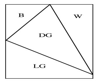
As in the C&M work, the particle tracks have different gradients; the gradients of the B-DG, W-DG, and LG-DG are, respectively, -1:1, 2:1, and -1:2. The LG-W boundary which would develop if there were more white cells is vertical.
