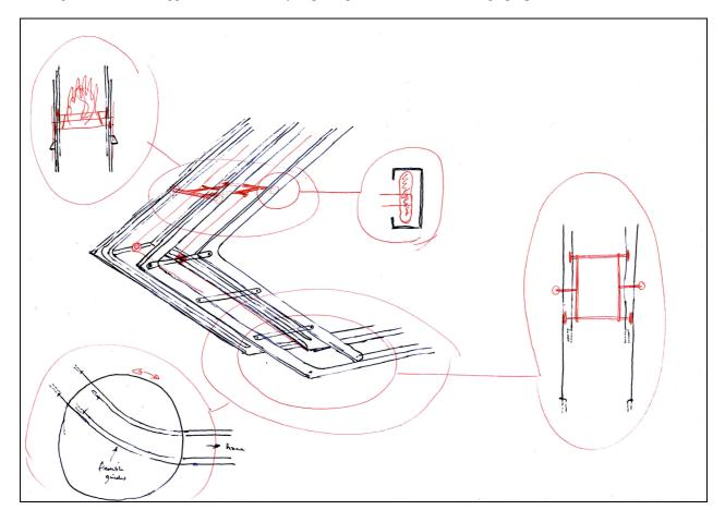
In accordance with the earlier discussion, it's modelled on an escalator-like<sup>3</sup> mechanism, with a carriage running on front and back "rails". The "rails" must enclose the wheels, as in the central inset, because the wheels must be able to run when the rails are turned over – consider bending the upper part of the arm as illustrated upwards through the vertical and on to a position in line with the lower section.
