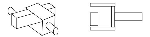
Now if the robot simply closes its gripper while keeping the horizontal effector carrying the gripper still, it could tear the handle off the door. It would be much better if it noticed when the bottom "finger" touched the handle, and adapted by moving the horizontal effector downwards while continuing to close the gripper until both "fingers" made contact. That's compliant motion.
