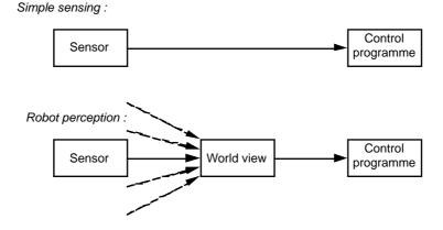
The world view is a representation of the robot's surroundings in the form of data structures of some sort. The nature of the representation, and the level of detail, can be whatever is suitable for the application; world views range from solid volume element models which record only whether each element is occupied or free to highly structured representations in which individual items are identified.
