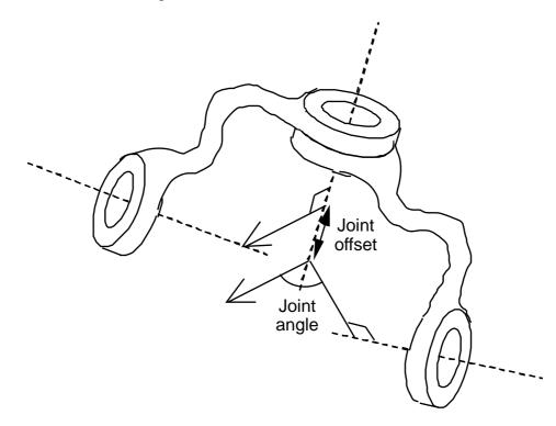
The four parameters – link length and twist, and joint angle and offset – are sufficient to define the configuration of a simple kinematic chain. Knowing these parameters and the position and direction of the base of a robot, one can work along the chain through links and joints as they appear, and calculate the position of the end of the chain.
