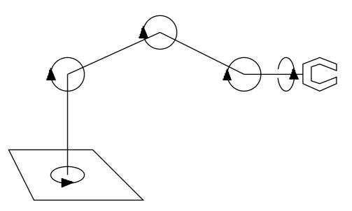
That robot has five degrees of freedom; some also provide means for varying the angle between the gripper axis and the final link in one or two directions (pitch and yaw).
