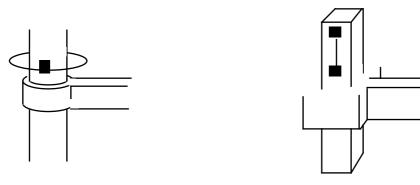
The state of each joint can be defined by giving a single coordinate, which measures the displacement ( distance or angle ) of the motion from some arbitrary standard position.
