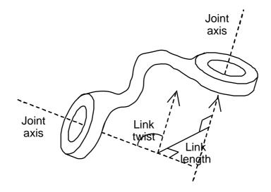
Notice that the two link parameters, link length and link twist, are independent of the curious shape of the link itself, and depend only on the relative position and orientation of the two joint axes which the link connects.
