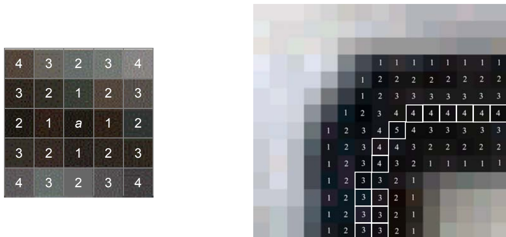
Figure 5 Pixel distances to pixel a (left) and the shortest distances to contour pixels (right)
