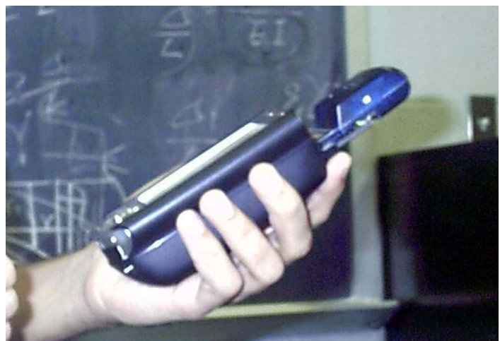
Figure 3 Client: iPAQ 3850 , GPS and Wireless Card
