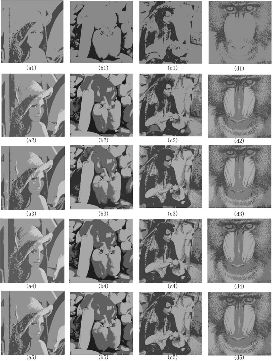
**Fig. 7.** Three-level thresholding images obtained by different methods. (a1)–(d1) K-means; (a2)–(d2) DE; (a3)–(d3)DEPS; (a4)–(d4)MIPSO; (a5)–(d5)MIPSOH.)
