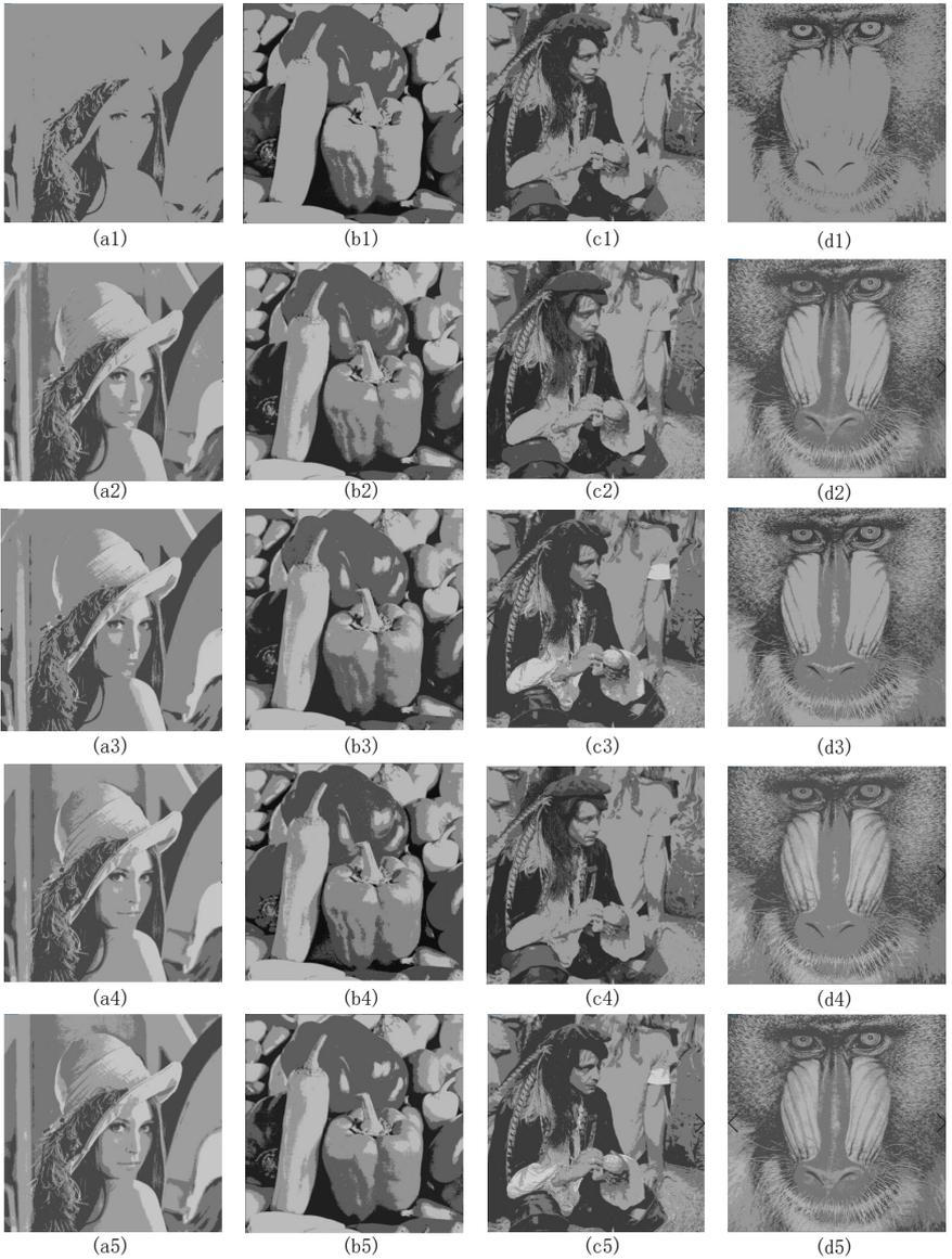
**Fig. 8.** Four-level thresholding images obtained by different methods. (a1)–(d1) K-means; (a2)–(d2) DE; (a3)–(d3)DEPS; (a4)–(d4)MIPSO; (a5)–(d5)MIPSOH.)
