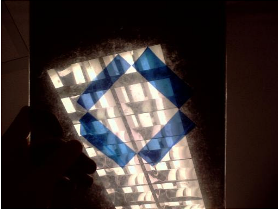
Fig. 4: Cellophane-based implementation. There are two layers of cellophane aligned perpendicularly. Where they overlap, both components of the phase are shifted the same amount, giving rise to an unobservable global phase shift.
