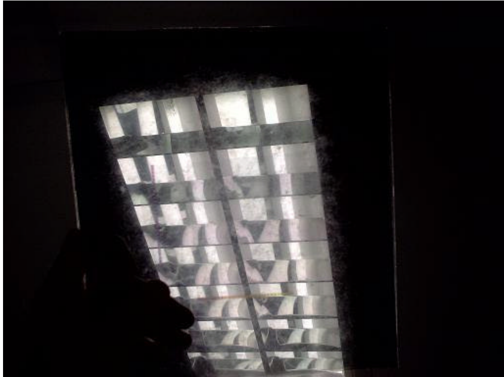
Fig. 5: Cellophane aligned with the polarizer, simulating classical inputs; we gain no information.
