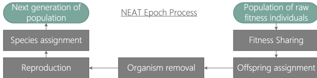
Figure 10: A model of the epoch process in more detail. The fitness sharing, offspring assignment and species assignment mechanisms are as those described previously in section 3.4. Reproduction mechanisms are those described in section 3.3.
