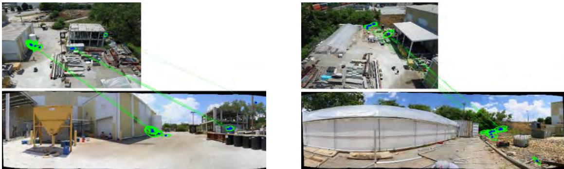
Fig. 9: Examples of the image matching results between UAV(upper) and UGV (lower) images
