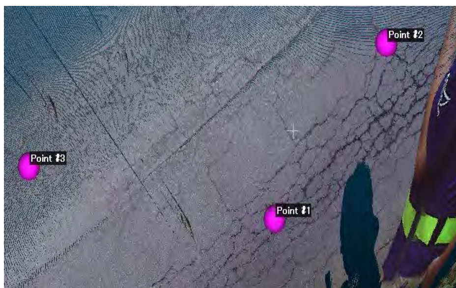
Fig. 7: Repair information linked with three-dimensional point cloud data.
