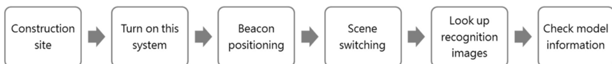
Fig. 6: Application process for presenting 3D model of BIM component and its attribute information.
