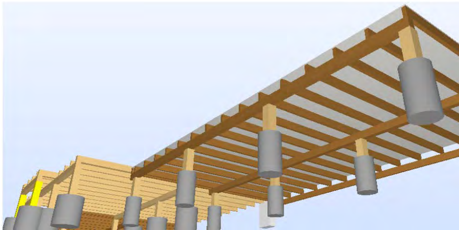
Fig. 3: Model view with a specific sub system selected (sub floor framing).
