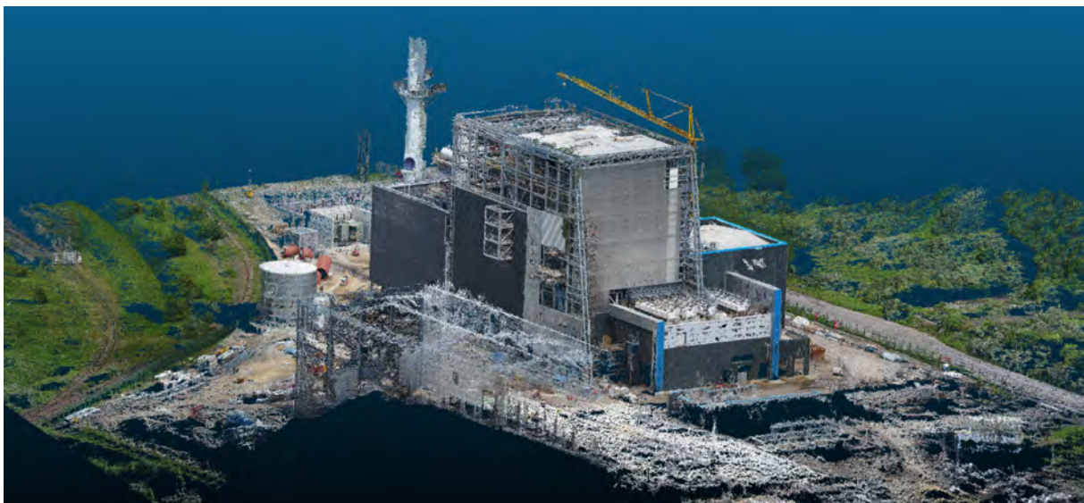
Fig. 6: Resulting point cloud model for the facility
