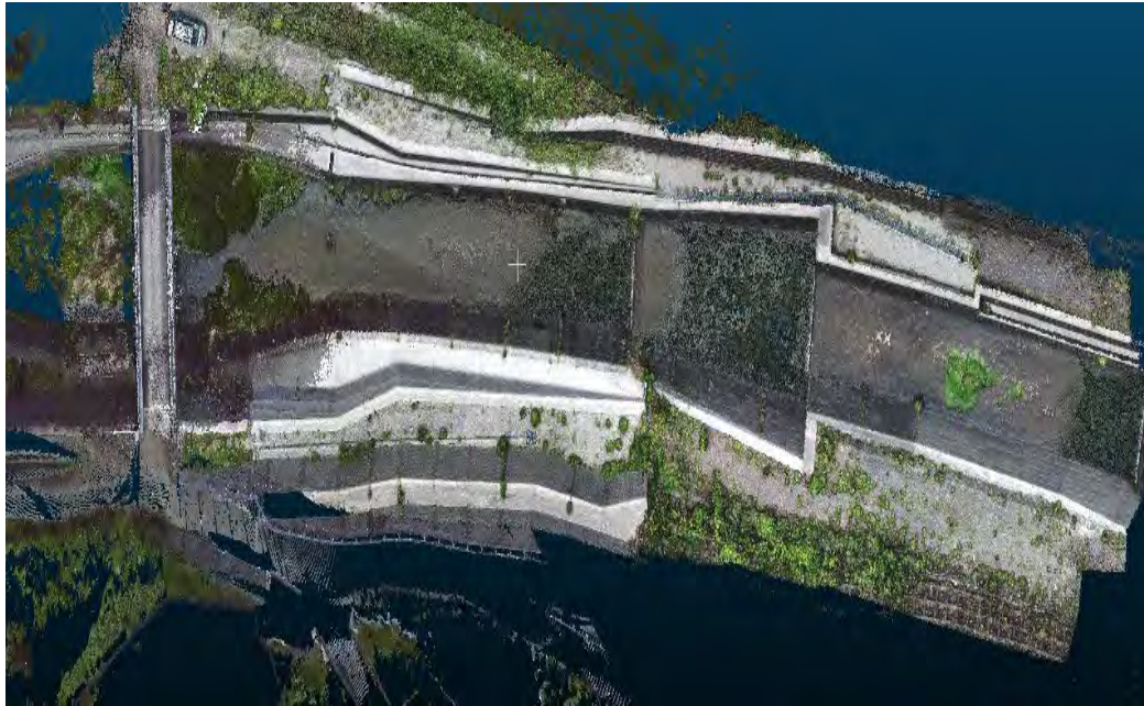
Fig. 4: Data fusion of TLS and UAV in road and river space.
