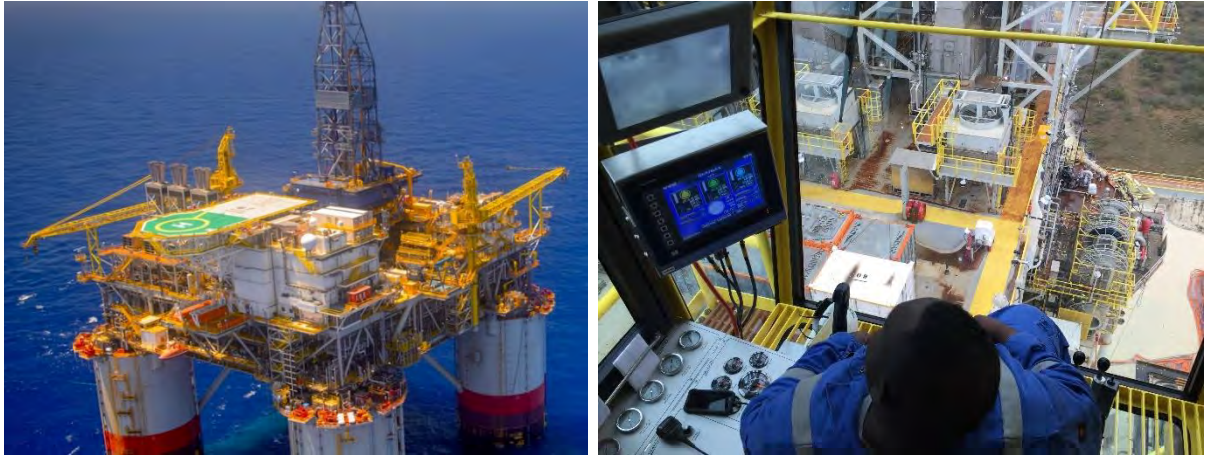
Fig. 1: Crane lift operations in offshore platform environment; Left image: two pedestal-mounted lattice boom cranes on an offshore platform (Chevron 2018); Right image: cab view from one of the cranes (image by Yihai Fang).
