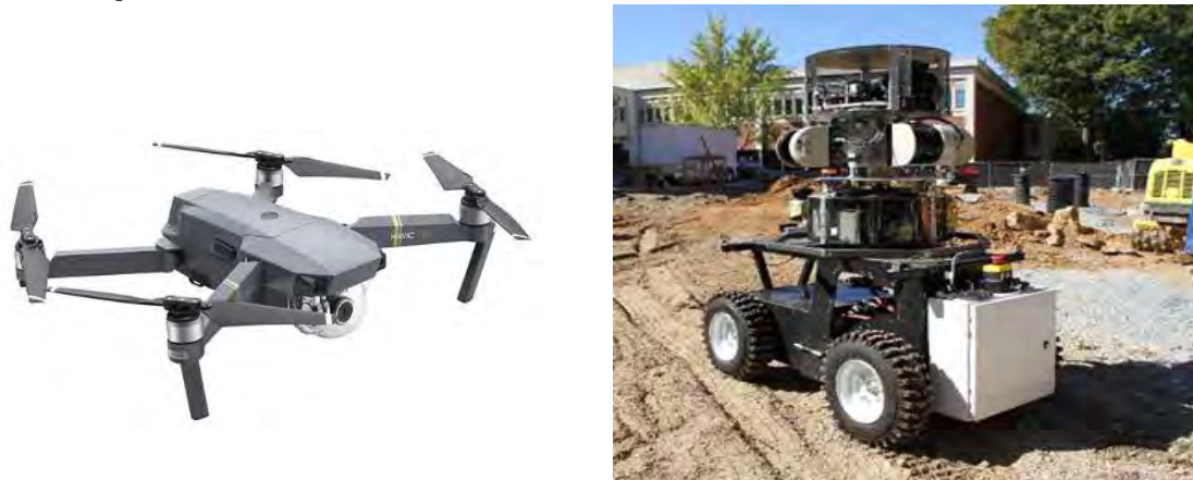
Fig. 6: The DJI Mavic Pro (left) and UGV (right) used in this research
