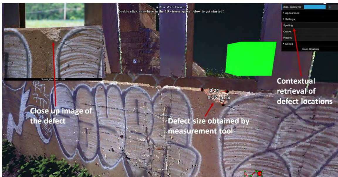
Fig. 5: Figures showing geotagging and measurement annotation tools within the immersive environment
