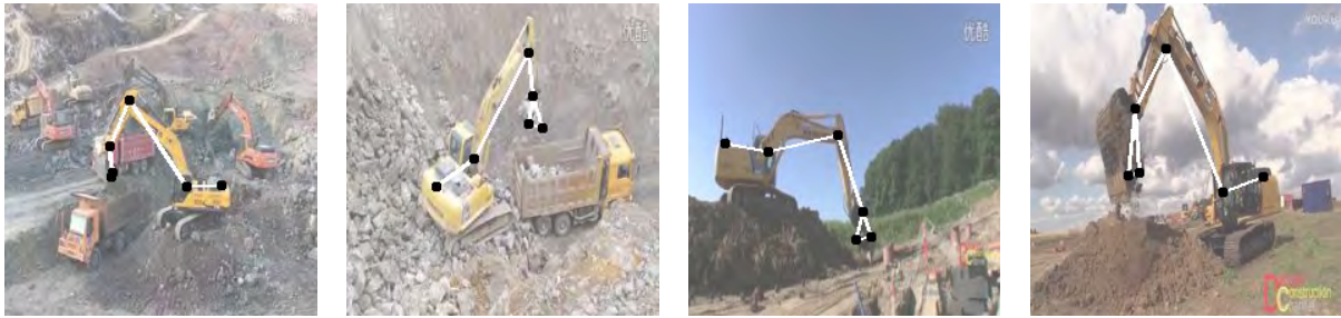
Fig. 5: Examples of construction equipment posture estimation results.
