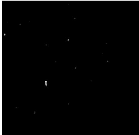
Fig. 8: A gaze heatmap Render Target texture in Unreal Engine 4. The white spots represent the area that was observed by the user. This would be translated into colored heatmap in the 3D environment.
