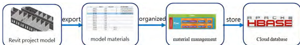
Fig. 2 : The process of exporting and storing Revit Model information.
