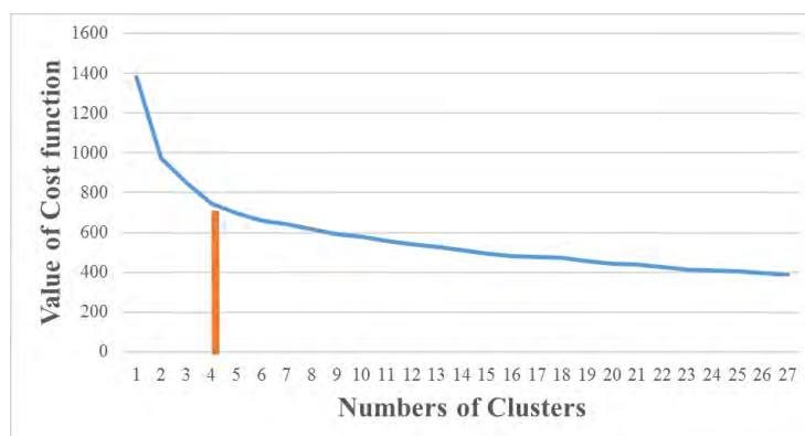
Figure 2 Determining number of clusters ( k )
