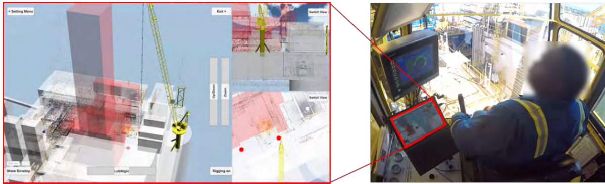
Fig. 6: Monitor cabin setup and user interface for real-time visualization
