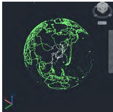
Fig. 5: View of world borders upon GRS80 surface using ECEF coordinate system.
