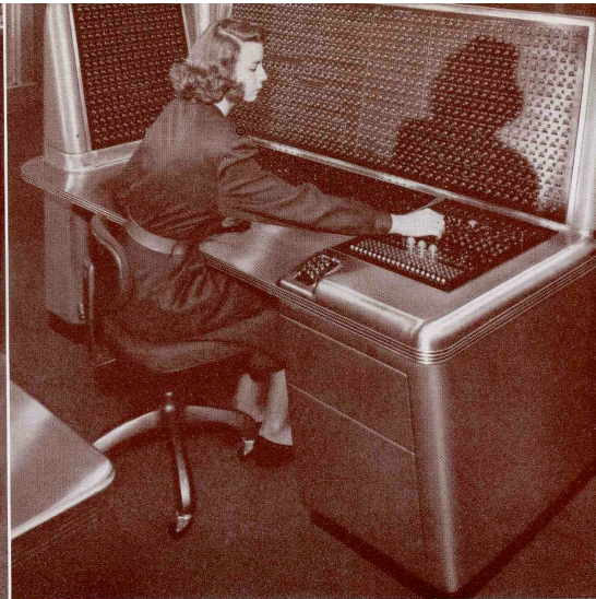
Console, or operation indicator and control desk.
