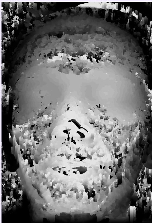
Depth map without structured lighting
