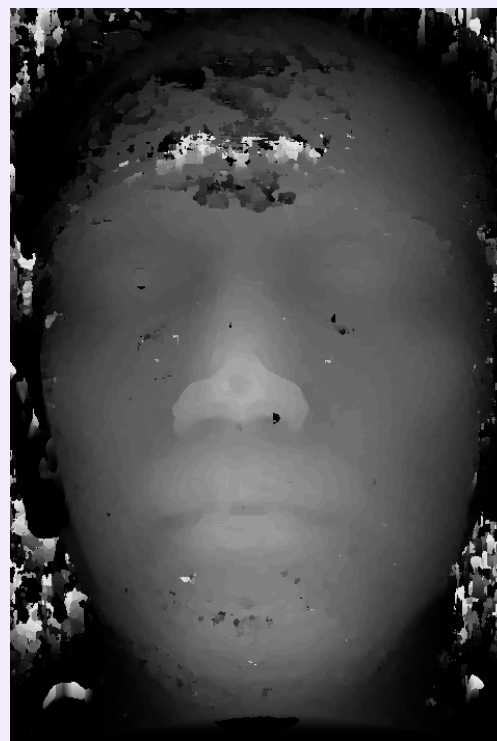
Depth map with structured lighting
