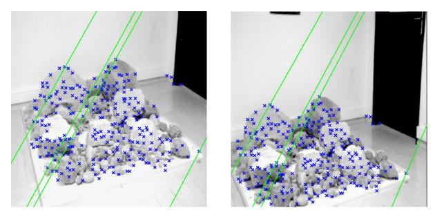
Fig. 8. Epipolar geometry estimated with the nonlinear method
