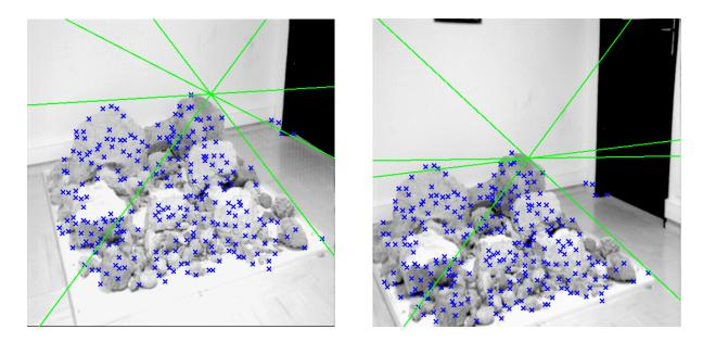
Fig. 6. Epipolar geometry estimated with the linear method
