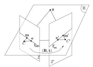
Fig. 1. The epipolar geometry
