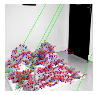
Fig. 5. Epipolar geometry estimated through classical stereo calibration, which serves as the ground truth
