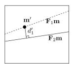
Fig.~10. Definition of the difference between two fundamental matrices in terms of image distances
