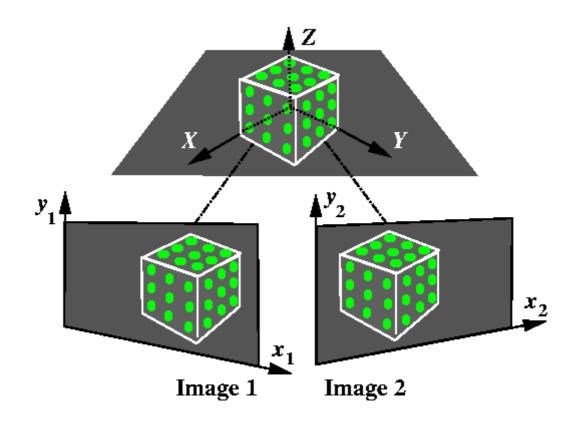
Your first task is to use the 3D calibration cube (**you <u>may</u> design a new calibration object**) to compute the intrinsic and extrinsic parameters of the calibration matrix for each camera. You will write an interactive program that collects data from your calibration object, the image plane, perform the calibration and output the calibration matrices and parameters. You must also evaluate the accuracy of the calibration.
