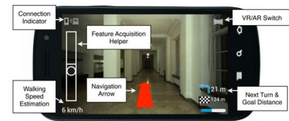
Figure 2. An environment which displays an augmented arrow. Arrow act as the navigation information.
