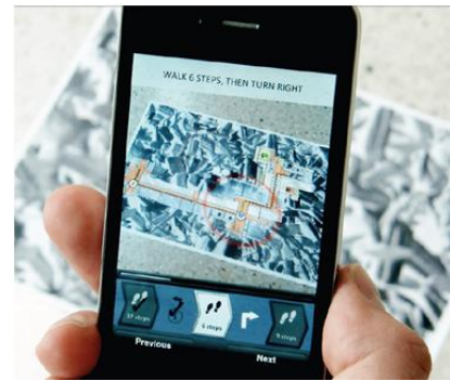
Figure 1. An image of the augmented reality interface which shows a WIM view of navigation space.
