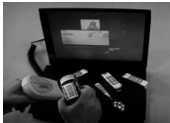
Figure 3. Various objects were RFID marked, and can be scanned by a bar code reader to display a scene of the story (Using the Every Object Tells a Story “memory chipped” devices [6])
