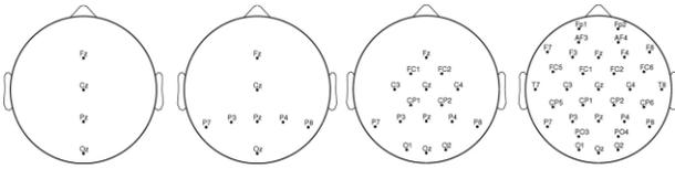
**Figure 1: Electrode configurations used in the experiments: Configuration I (4 electrodes), Configuration II (8 electrodes), Configuration III (16 electrodes) and Configuration IV (32 electrodes) [5]**
