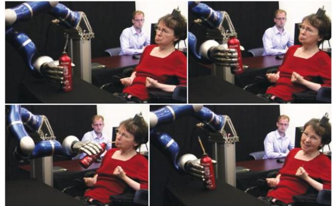
**Figure 2. Participant with an ECoG device connected directly to her brain is drinking from a bottle using the DLR robotic arm. [4]**
