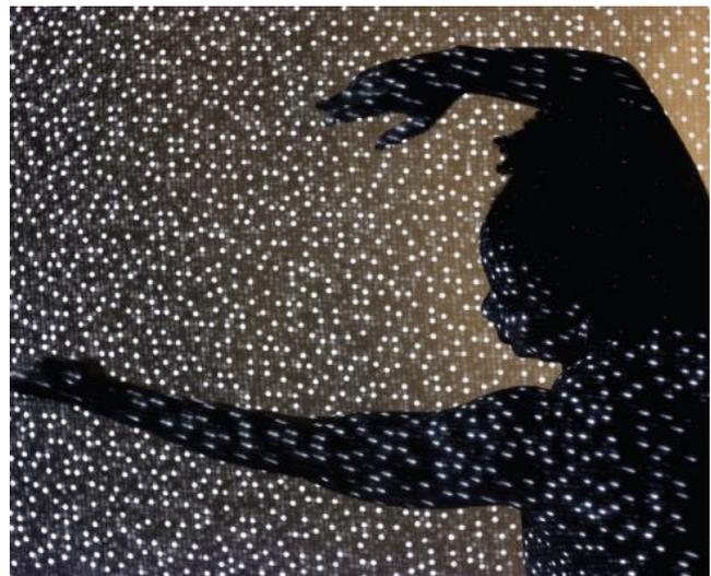
Figure 2: Kinect's infrared structured light[7]
