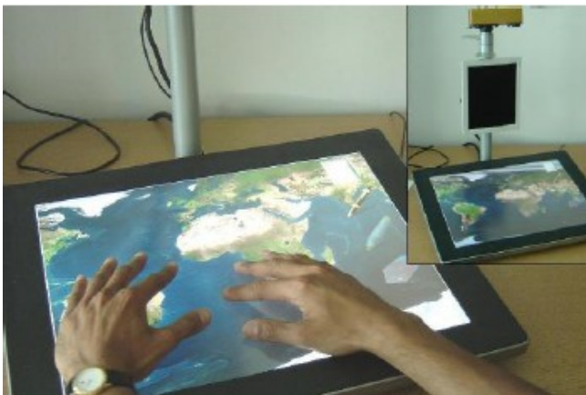
Figure 3: Set up for multi-touch using overhead cameras[1] This paper [1] advocates a different approach to multi-touch interaction that does not use FTIR.
