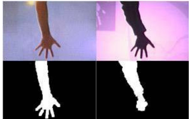
Figure 2 The images at left are the raw and processed hands using polarizing filters and skin detection. The images at right display RGB tracking without polarizing filters.[2]
