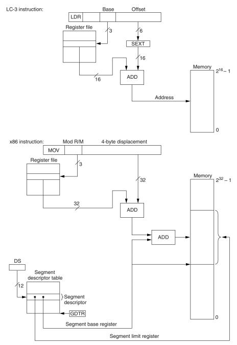
Figure B.2 Register+offset addressing mode in LC-3 and x86 ISAs
