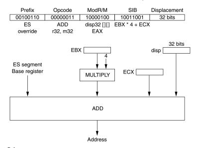
Figure B.6 Addressing mode calculation for Base+ScaledIndes+disp32
