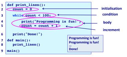
**Initialisation**: anything which needs to be done before the loop starts. **condition**: a boolean expression which is tested repeatedly to determine whether the body of the loop should be executed or not.
