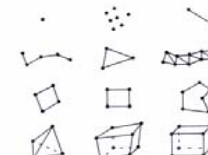
(f) Unstructured Grid (vtkUnstructuredGrid)
