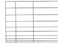
(b) Rectilinear Grid (vtkRectilinearGrid)
