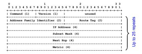
Get used to this form of protocol data unit drawing – it's how all basic Internet standards show bits and bytes. This shows 24 bytes in 6 rows of 4 bytes.
