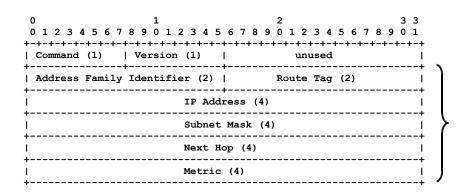
Get used to this form of protocol data unit drawing – it's how all basic Internet standards show bits and bytes. This shows 24 bytes in 6 rows of 4 bytes.
