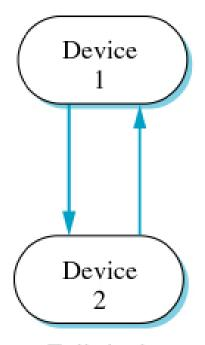
Full-duplex communication can go both ways simultaneously.
