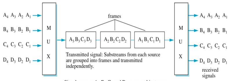
Signal sources:  $A_i$ ,  $B_i$ ,  $C_i$ , and  $D_i$  represent bit streams.
