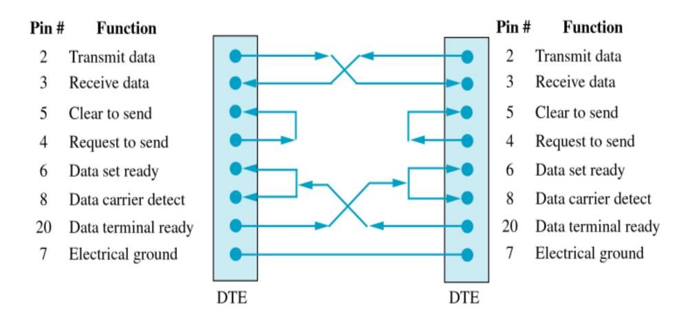
Not shown here: pin 22 = Ring Indicator, pin 1 = Protective Earth
