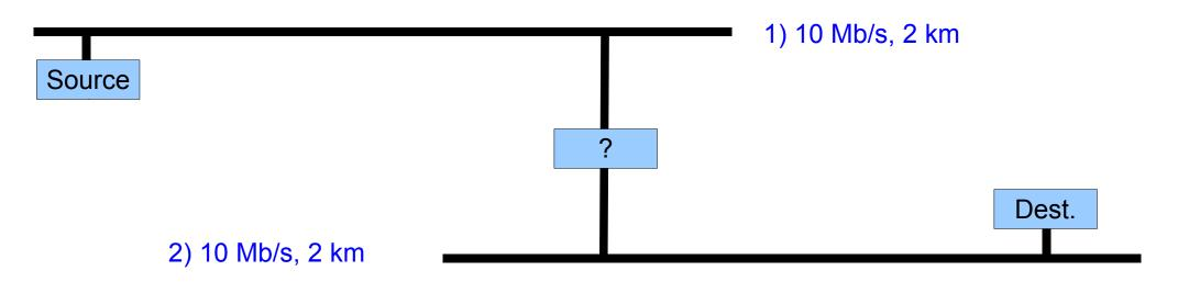
What must we do to avoid joining the two collision domains into one?
