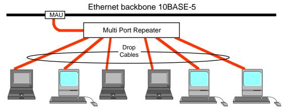
The Repeater provides several ports (often 8) each looking like an MAU, and has a single "device" port to allow connection to an MAU on the cable. The repeater detects collisions on "its" devices and from the cable. It passes appropriate collision signals back to the devices and a jam to the cable. The result is that all devices see standard Ethernet and follow Ethernet protocols, but there is only one connection to the cable.
