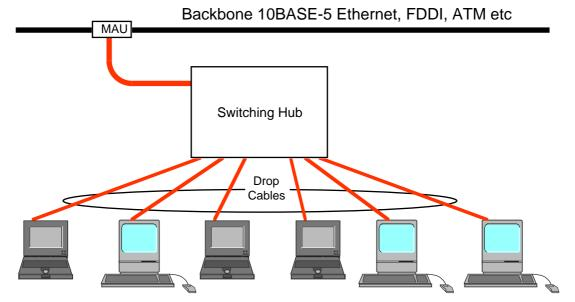
Traffic to another idle port may be forwarded immediately, but traffic to a busy port or to the backbone may be buffered until it can be sent. A collision may be signalled if no buffers are available or if the destination is unavailable. Even though the switching hub often contains buffers for each port, the ports still operate under standard Ethernet protocols as far as the user is concerned. The "collision" indication just signals that information cannot be accepted just then.
