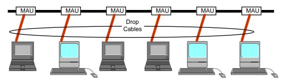
A problem in a laboratory or other large concentration of computers is that a long cable may be required just to fit the necessary MAUs. The cable is not very flexible and it may be difficult to fit the necessary length into a room. It is also easy to exceed the the cable length and/or the number of physical connections to the cable.
