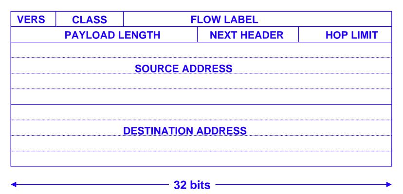
note: no header checksum, payload length doesn't include basic header, next header gives type of the header that follows, time to live replaced with real hop limit.
