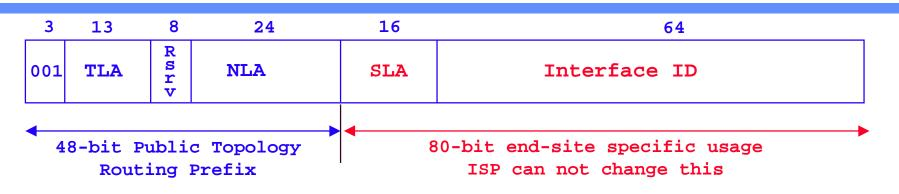
**TLA** = Top-Level Aggregation ID - are assigned to ISPs and Exchanges that act in a default-free way with a routing table entry for every active TLA ID (this constrains the routing complexity)
