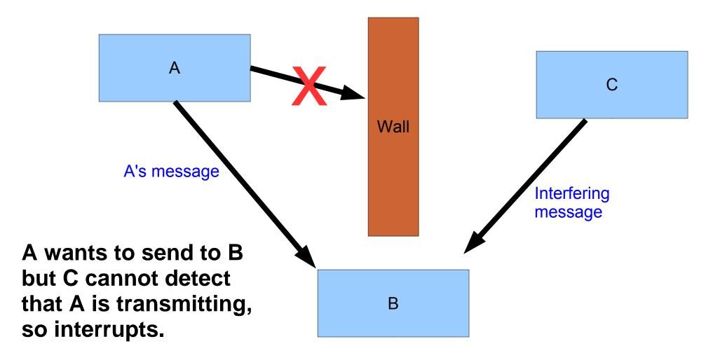
Solution: A and B exchange short "request to send" and "clear to send" packets. C missed the RTS but hears the CTS and keeps quiet. (Optional and not found on cheaper equipment.)
