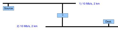
What must we do to avoid joining the two collision domains into one?
